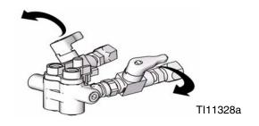
2. Connect A (ISO) and B (RESIN) fluid hoses to fluid manifold.
